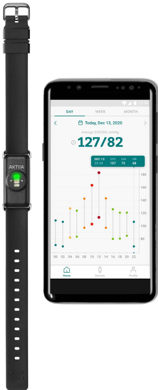
Aktiia Bracelet and the associated smartphone application to visualize SBP and DBP. DBP, diastolic blood pressure; SBP, systolic blood pressure.
